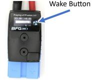
after the 'Wake' button is pressed. Pressing the 'Wake' button again will cycle the display through various pages
