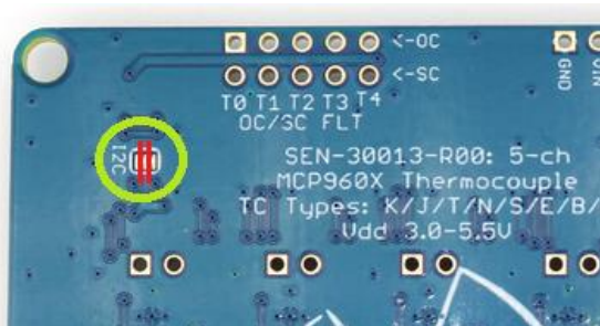
Figure 1 - Location of I 2 C pull-up cuttable trace
