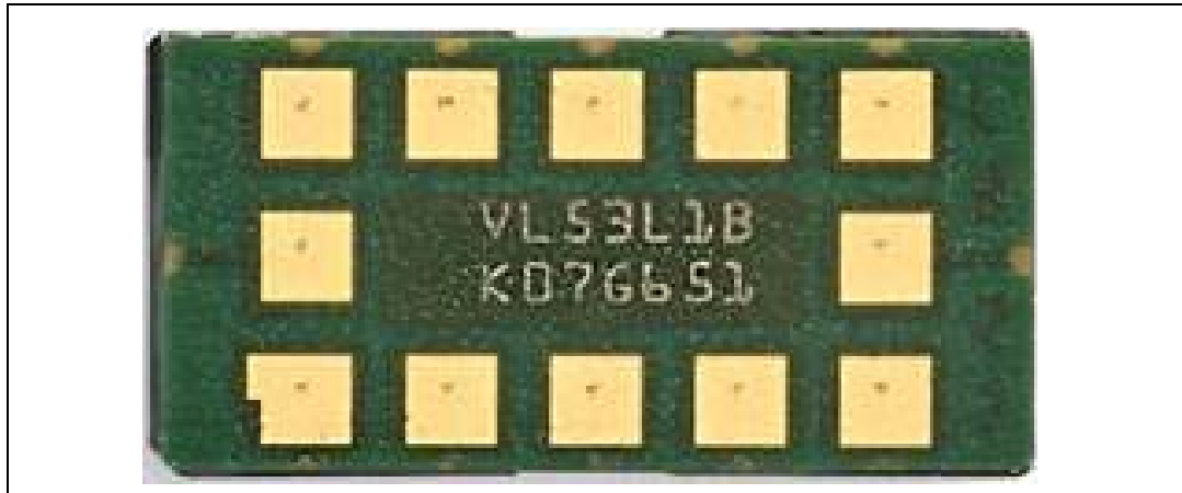
Figure 22. Example of prototype marking
