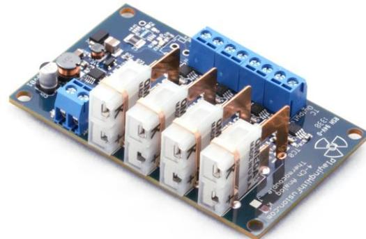
designed to support a wide variety of applications, from hobbyist projects (Arduino, homebrew) to automotive and industrial temperature measurement. See Table 1 for the optimized operating range for the different sensor options.
