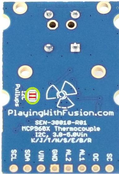
Application: one pair of pull-up resistors are required for proper I2C operation. If multiple breakouts are used together (think Qwiic daisy-chain), it is possible that an excessive amount of resistance can cause bus issues. If this is the case, resistance must be removed from one or more devices. SEN-30010 has cuttable traces on the back side of the board to make this easy.
