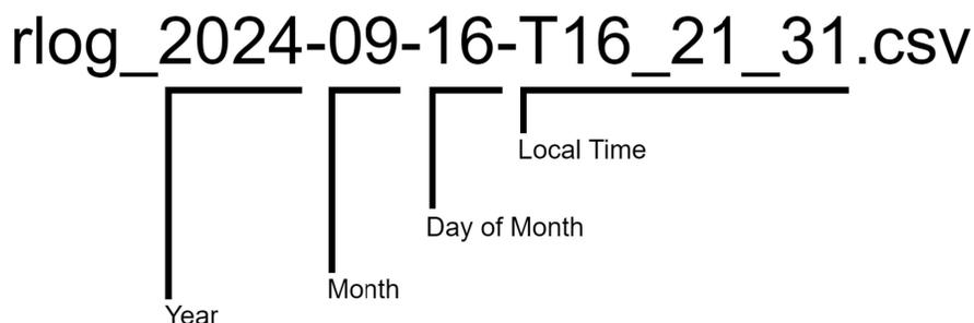
Figure 10: R3aktor Control Center Log File Format
