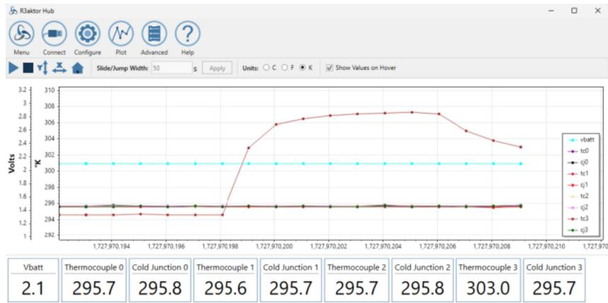
Figure 2: A connected R3aktor logging 4 channels of TC data and the VBatt
