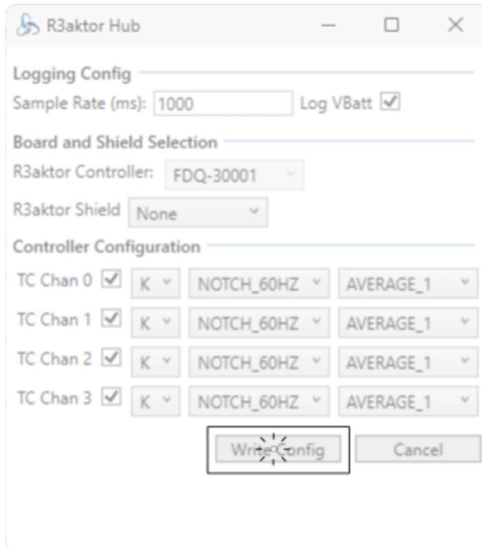
Figure 5: Writing configuration to connected R3aktor board
