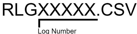
Figure 11: R3aktor Core Log File Naming Format
